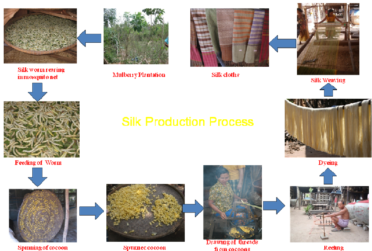
Figure 4: Silk production process.
