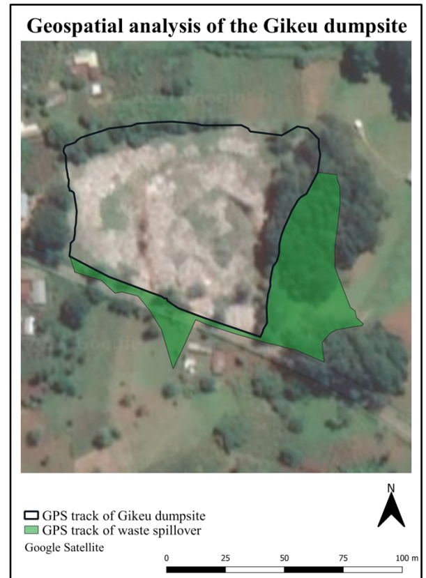
Figure 4.1. Map of Gikeu dumpsite showing the GPS track of the dumpsite and waste spillover. The geodata were used to measure the area (km 2 ). The map was produced in OGIS.
