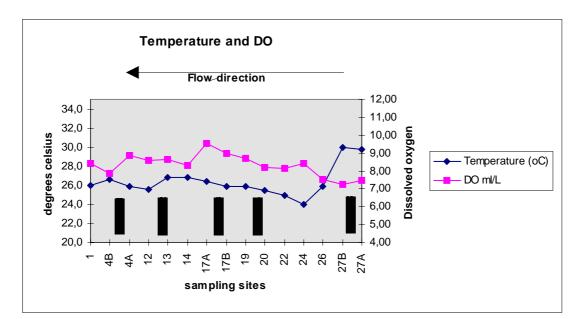
Graph 1: Temperature and Dissolved Oxygen from upstream to downstream
