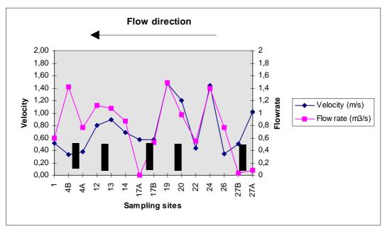
Graph 5: Velocity and flow rate Upstream-Downstream
